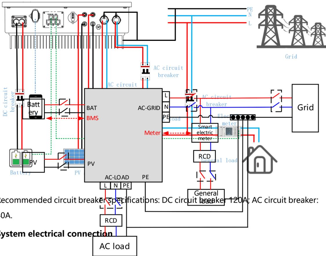
Recommended circuit breaker specifications: DC circuit breaker 120A; AC circuit breaker: 40A.
