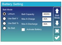
**Battery capacity:** it tells hybrid inverter to know your battery bank size.
