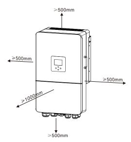
For proper air circulation to dissipate heat, allow a clearance of approx. 50cm to the side and approx. 50cm above and below the unit. And 100cm to the front.
