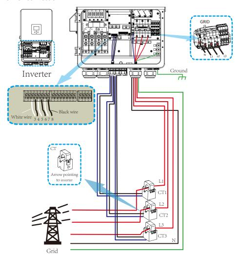
\*Note: when the reading of the load power on the LCD is not correct, please reverse the CT arrow.
