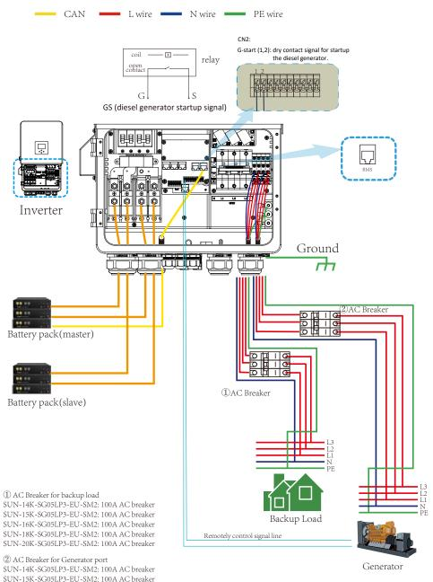
SUN-16K-SG05LP3-EU-SM2: 100A AC breaker SUN-18K-SG05LP3-EU-SM2: 100A AC breaker SUN-20K-SG05LP3-EU-SM2: 100A AC breaker
