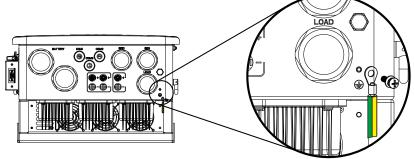
Earth connection (Copper wires)
