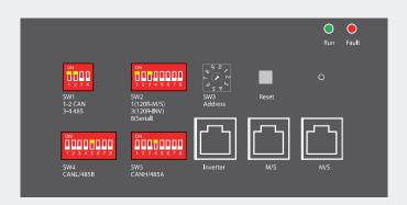
For Parallel connection, SW2 DIP 8 select 'OFF' For Series connection, SW2 DIP 8 select 'ON '
