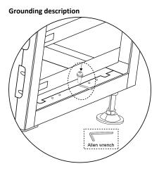
Twist one end of the ground wire harness (8) in 4.8 to the wiring position shown in the figure, and twist the other end to the ground copper bar of the PDC using an Allen wrench.
