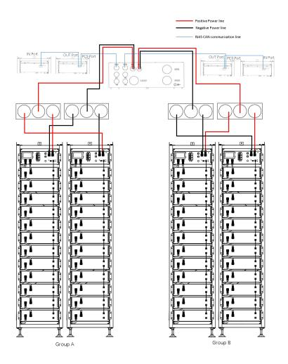
The number of battery packs in group A or Group B must be the same. The number of battery packs in group A and group B can be different.
