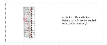
1. After the battery module is placed in the control box, take out a 140 mm communication cable to connect the communication port of the battery module and the high-voltage control box, and 11x110mm communication cables to connect the battery module communication port (IN-OUT) from top to bottom. (12 communication cables in total).
