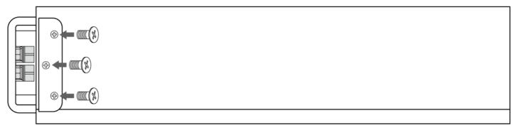
3. Fix two wall-mounted brackets onto the wall with 4 expansion bolts (M6\*100).
