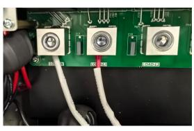
Step 5:Complete the wiring and conduct the inspection..
