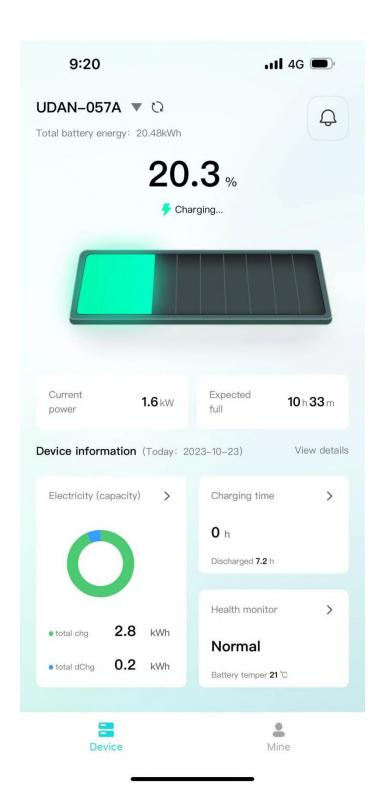
• The top area displays the device name, battery energy, and message entry.
